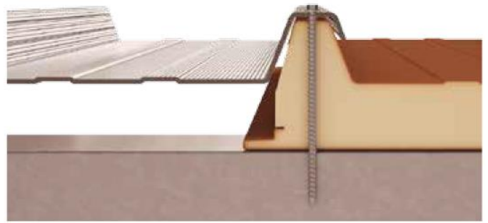
Fixing of the translucent corrugated sheet on the corrugated panel.
