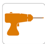
PORTABLE DRILL twist bit max 8 mm Ø
